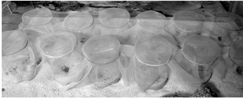
Fig. 2. Experimental setup showing the saltwater aquarium containing twelve bottled chambers with netted tops.
